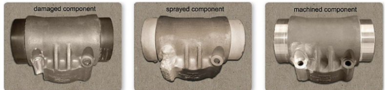
Restoration process of a mechanically damaged flap transmission tee box housing of an aircraft via CSAM
