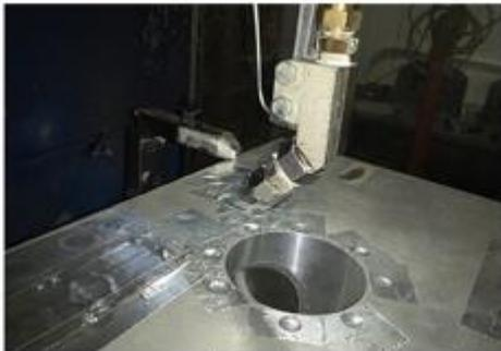
Fig. 4 Experimental setup to repair the valve actuator with internal bore nozzle
