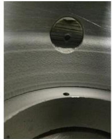
Fig. 17 Photo of bottom inside corner of the internal bore showing the lack of fill in the bottom corner during the initial deposition trials
